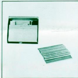
Lead Rules (metal stripes that are used to increase the space between lines)
